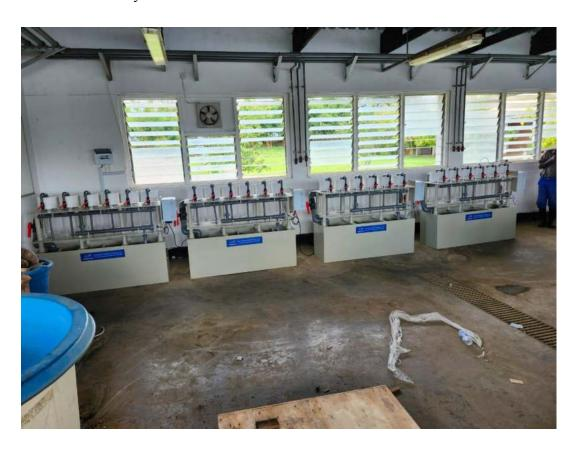
Photo 1: High-End Macdonalds Fish Egg Incubators installed at Bunda Fish Farm.
